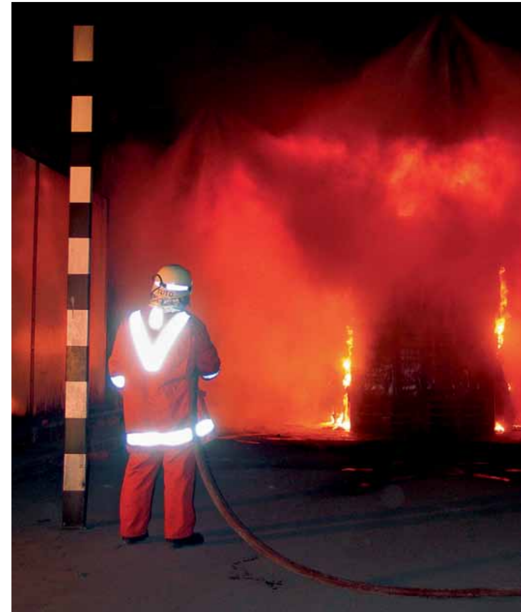
Full-scale fire test carried out for a tunnel project.
