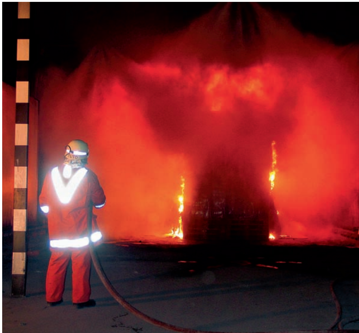
Full-scale tunnel fire test carried out for the M30 Madrid tunnel project.
